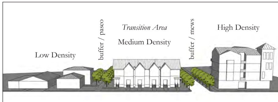
FIGURE 5-36: Transitions of development intensity from higher density development building types to lower can be done through building types or treatments that are compatible with the lower intensity surrounding uses. Boundaries can be established by providing pedestrian paseos and mews to create separation, rather than walls or fences.
