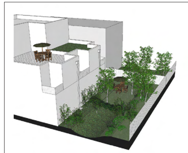
FIGURE 5-42: Minimize stormwater runoff to impermeable areas with landscaping, green roofs, and rain gardens when possible.
