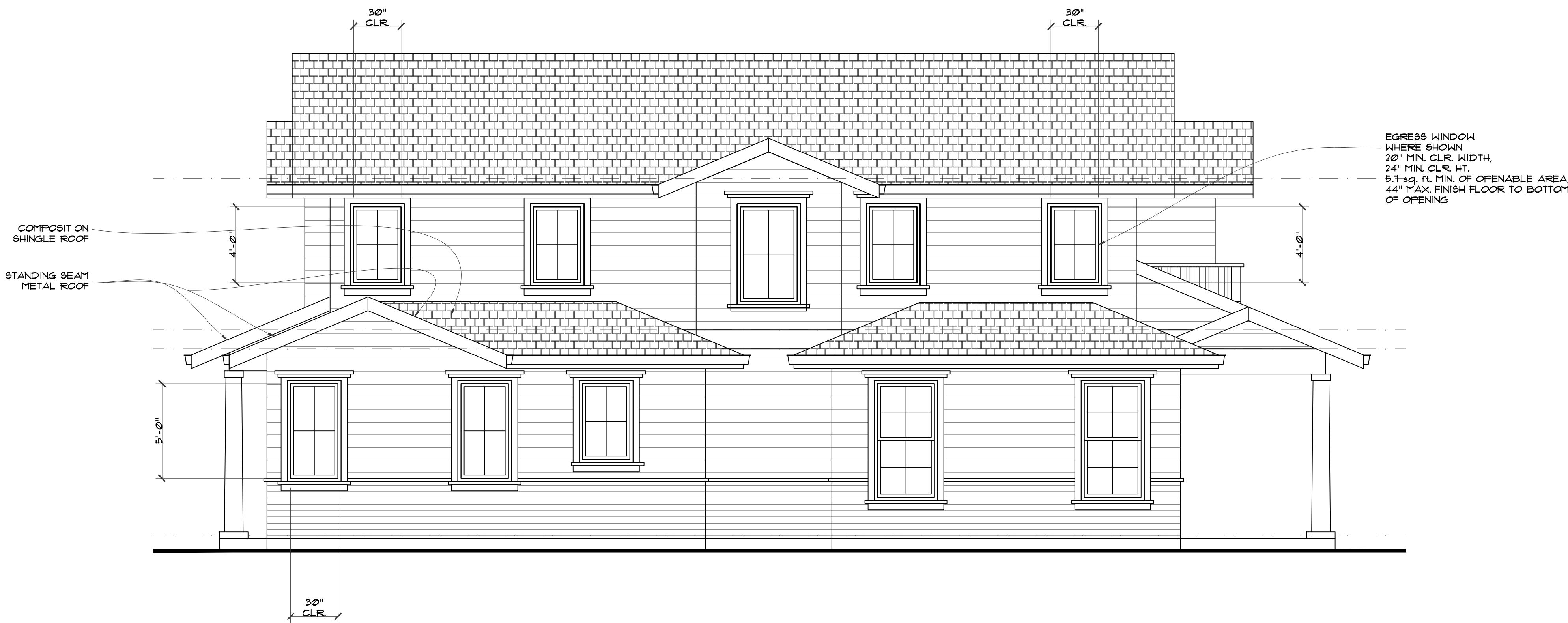
RIGHT-SIDE ELEVATION ( PROPOSED ) 1/4" = 1'-0"
