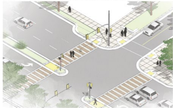
Figure 32: Illustrative Curb Bulbout if Bicycle Lane Present
