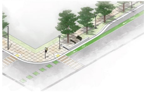
Figure 32: Illustrative Curb Bulbout if Bicycle Lane Present
