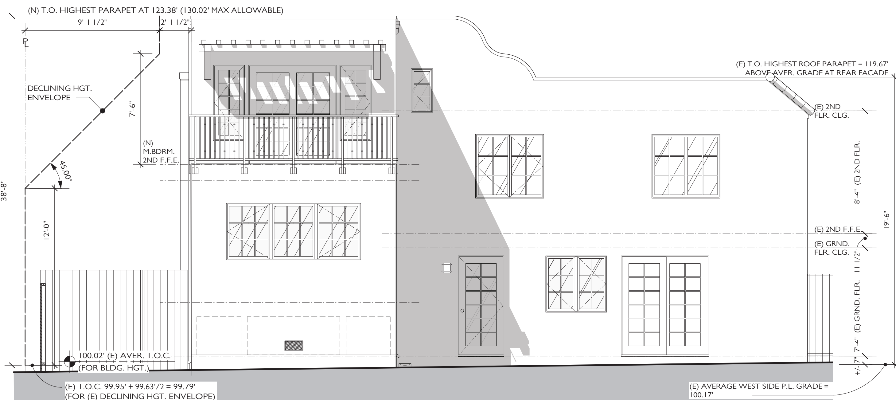
1 A0.1 NORTH (BACK) ELEVATION - PROPOSED Scale: 1/4" = 1'-0"
