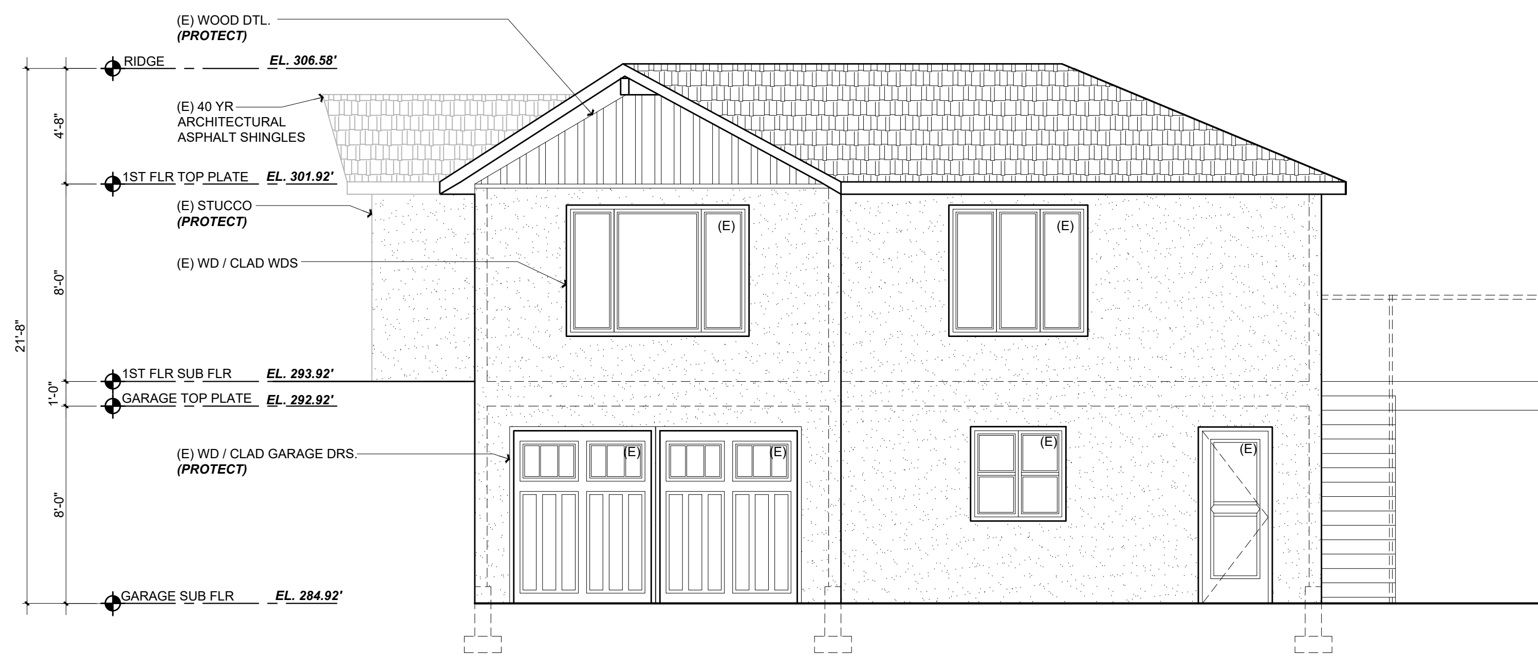
EXISTING RIGHT ELEVATION
