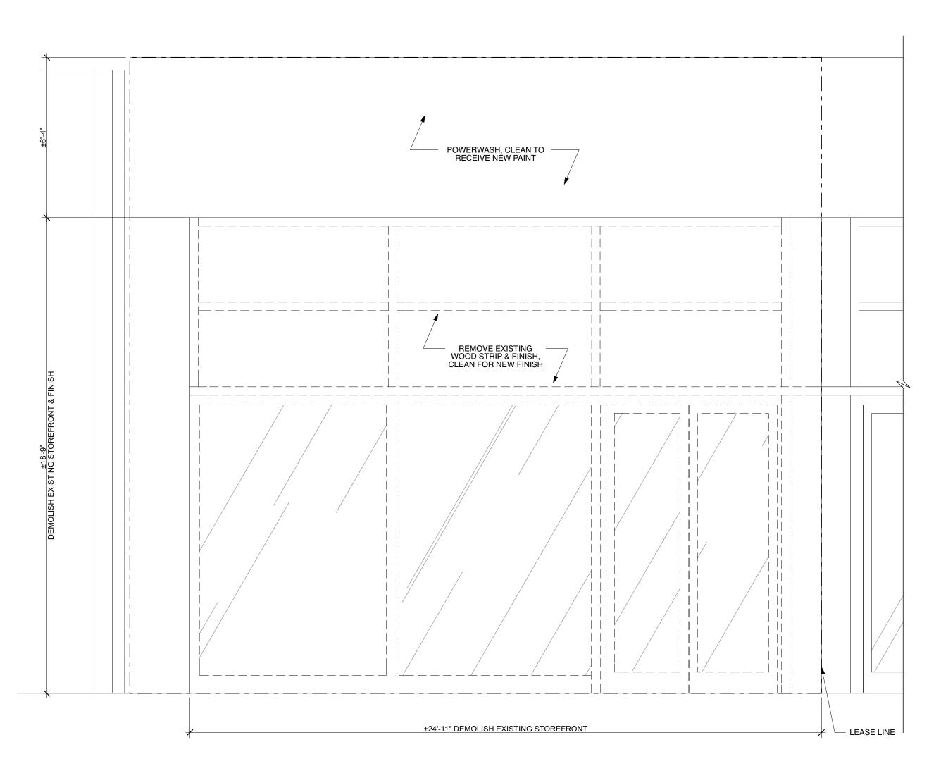
STOREFRONT ELEVATION - DEMOLITION SCALE: 3/8" = 1'-0"
