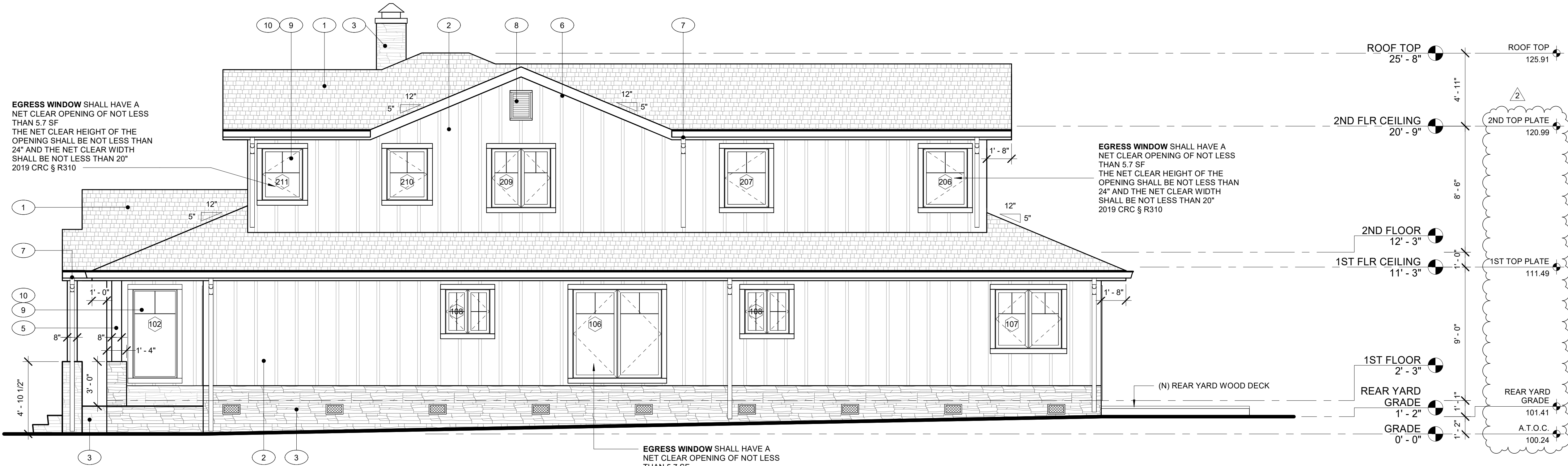
1 BUILDING NORTH ELEVATION - PROPOSED SCALE: 1/4" = 1'-0"
