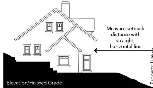
Figure 25.30-5: Setback Measurement for Sloped Lots
