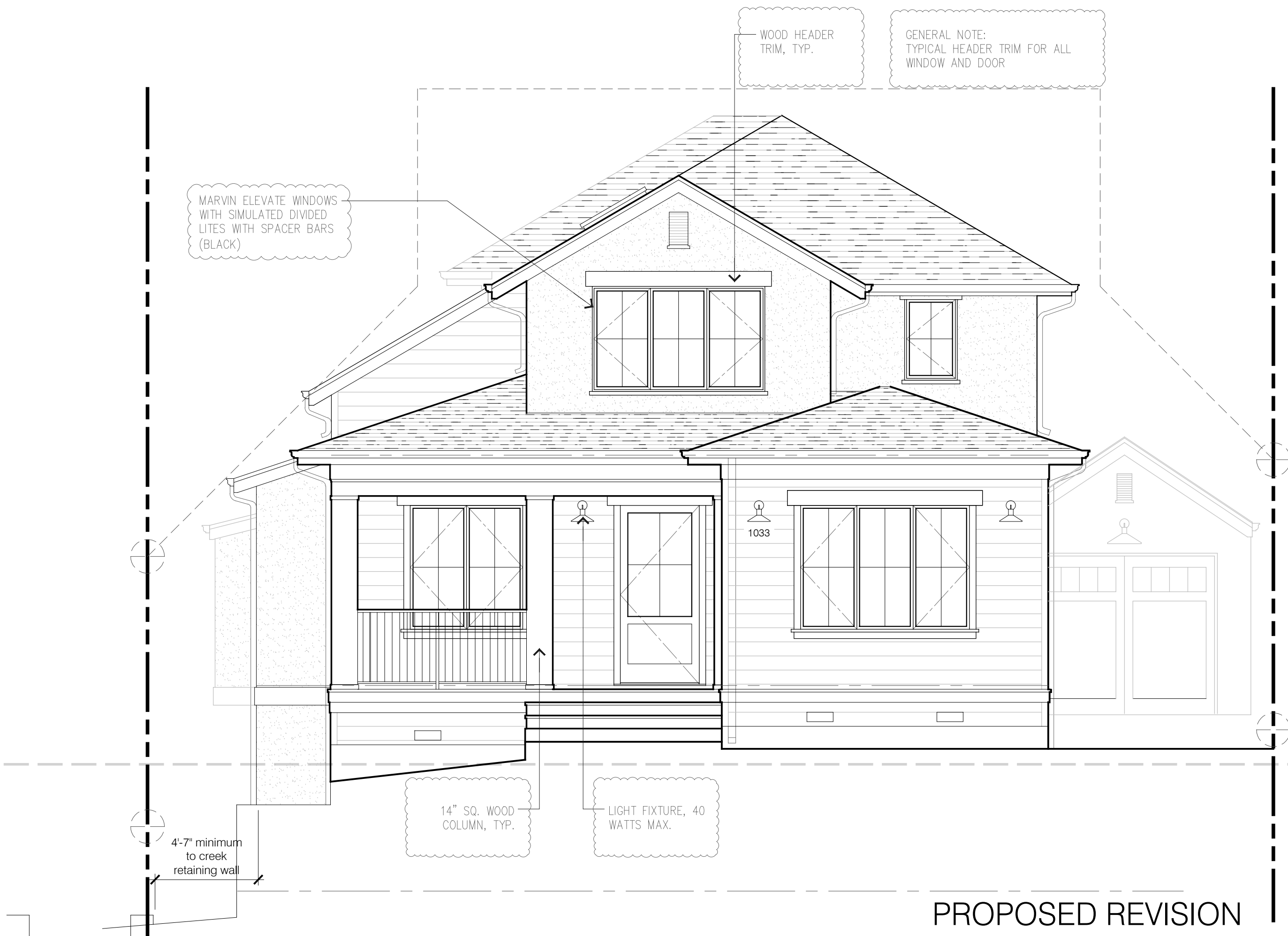
PROPOSED REVISION FRONT (NORTHEAST) ELEVATION
